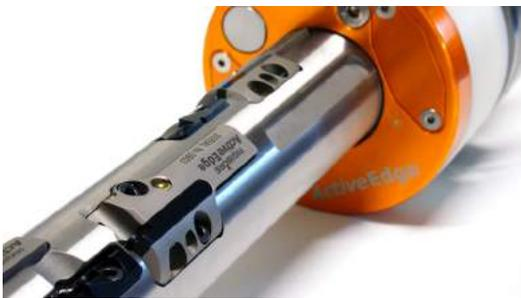
Each ActiveEdge cartridge is **independently adjustable**, based on data provided by in-process measurement as the tool wears.
