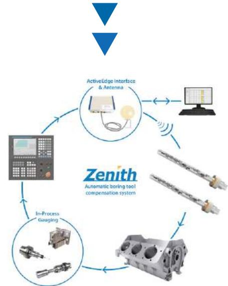
This closed-loop boring cycle allowed micron accurate cutting edge adjustments **without any operator intervention**.
