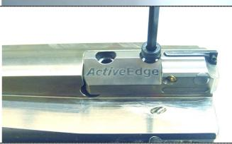
If the original cartridge has been re-fitted to the same pocket, use ActiveNet to carry out a tool status check to confirm the tool is ready for use.
