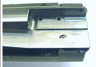
Fit the cartridge, ensuring that it is firmly seated on all 3 qualified pocket faces.
