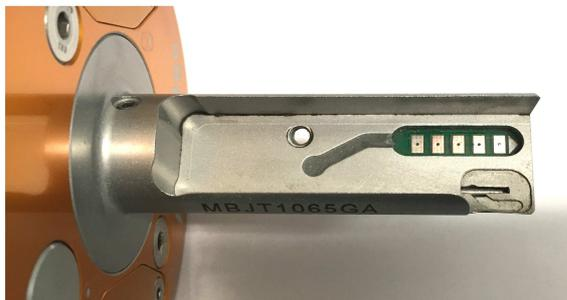
The cartridges are fitted to dedicated pockets with integral electrical contacts
