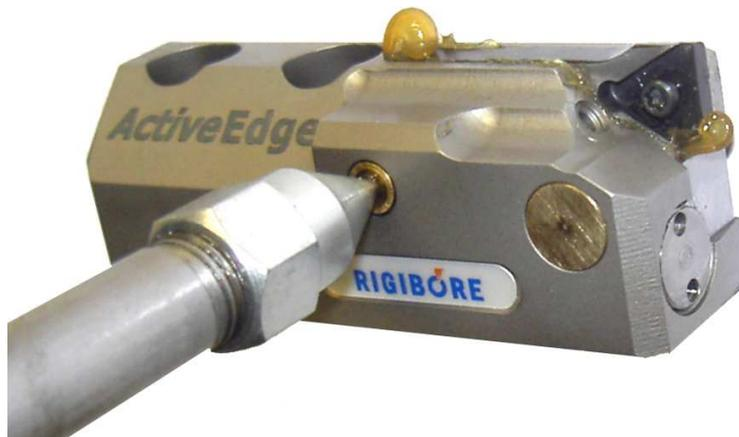
Castrol Longtime PD2™ grease should be used. A recommended grease gun and refills can be purchased from Rigibore.
