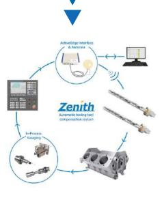
Each ActiveEdge cartridge is **independently adjustable**, based on data provided by in-process measurement as the tool wears.
